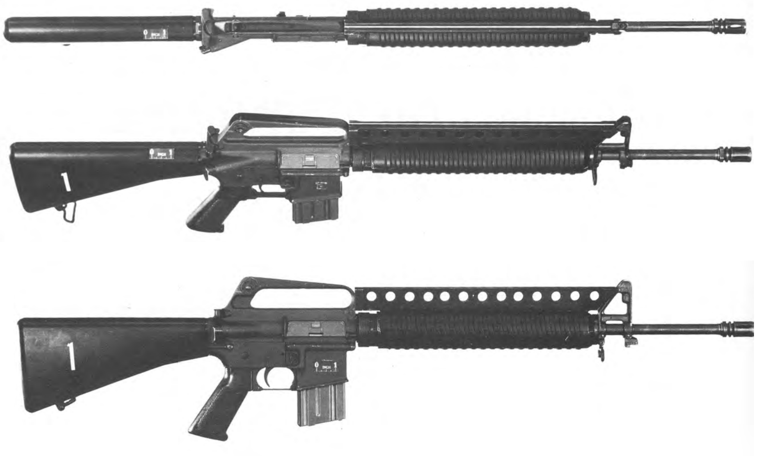
349. Three views of a special, experimental M16A1, designed by the Human Engineering Labs (HEL) for faster target acquisition. Note the highlighted, full-length sighting groove. Used in the SAW trials.
