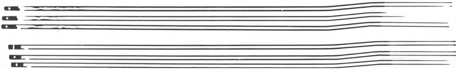
292. X-ray photograph of M16A1 test rifle gas tubes, showing fouling buildup after 2,000 rounds of M193 ball ammunition. Note that fouling produced by ball powder (WC846) is most noticeable and is concentrated near gas tube
