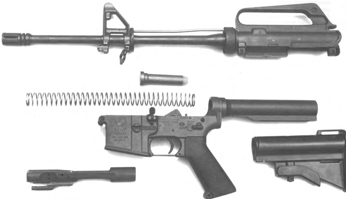
278. Left side view of a late Colt model 653 M16A1 Carbine (14.5" barrel) serial no. 9279755, partially stripped. Overall length (stock retracted): 29.8"
