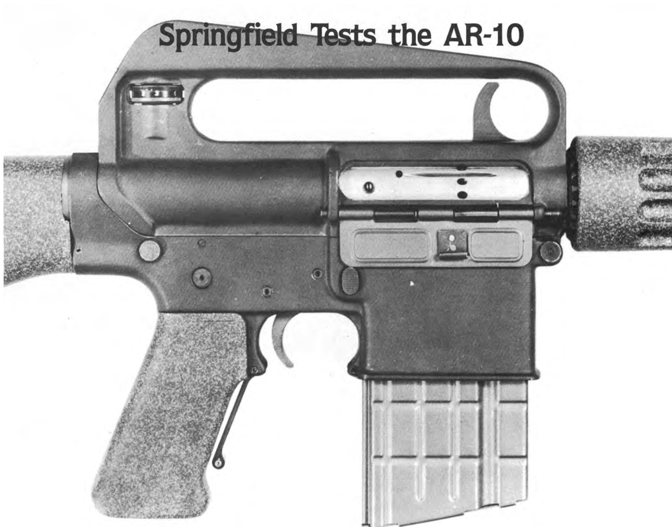
3& AR-10 serial no. 1004 action closeup, right side view. Note the winter triggerguard and early spring-clip dust cover latch.
