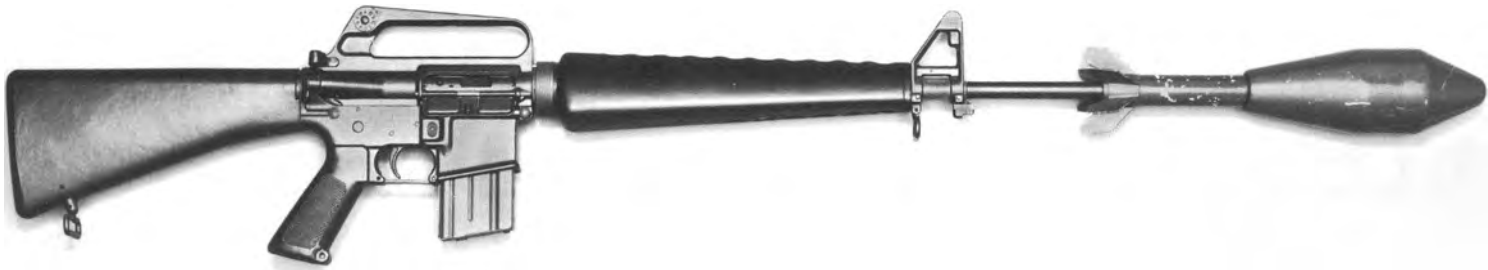
236. XM16E1 shown ready to fire an Energa-type rifle grenade. At Staff level, this concept of launching bulky grenades by means of dedicated grenade-blank cart-
