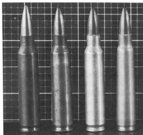
141. Evolution of the .223 cartridge. From left: 1. Gene Stoner's original un-headstamped "stretched" .222 Remington, loaded with his 55-grain bullet, identified as "Type B" in Frankford Arsenal's Investigation of Bullet Configuration report of June, 1963; 2. The .222 Remington Special, loaded with Remington's 55-grain 5.5-caliber tangent ogive bullet (the inferior "Type A" in the Frankford report), headstamped REM - UMC 222 SPL (fig. 76); 3. A typical M193 5.56mm round, (actually an inert, nickel-cased "Display" version of Fabrique Nationale's M193 counterpart) headstamped FN 75; 4. An interesting experimental "tapered case" .223 round by Fabrique Nationale, headstamped FN 68. Editor's collection
