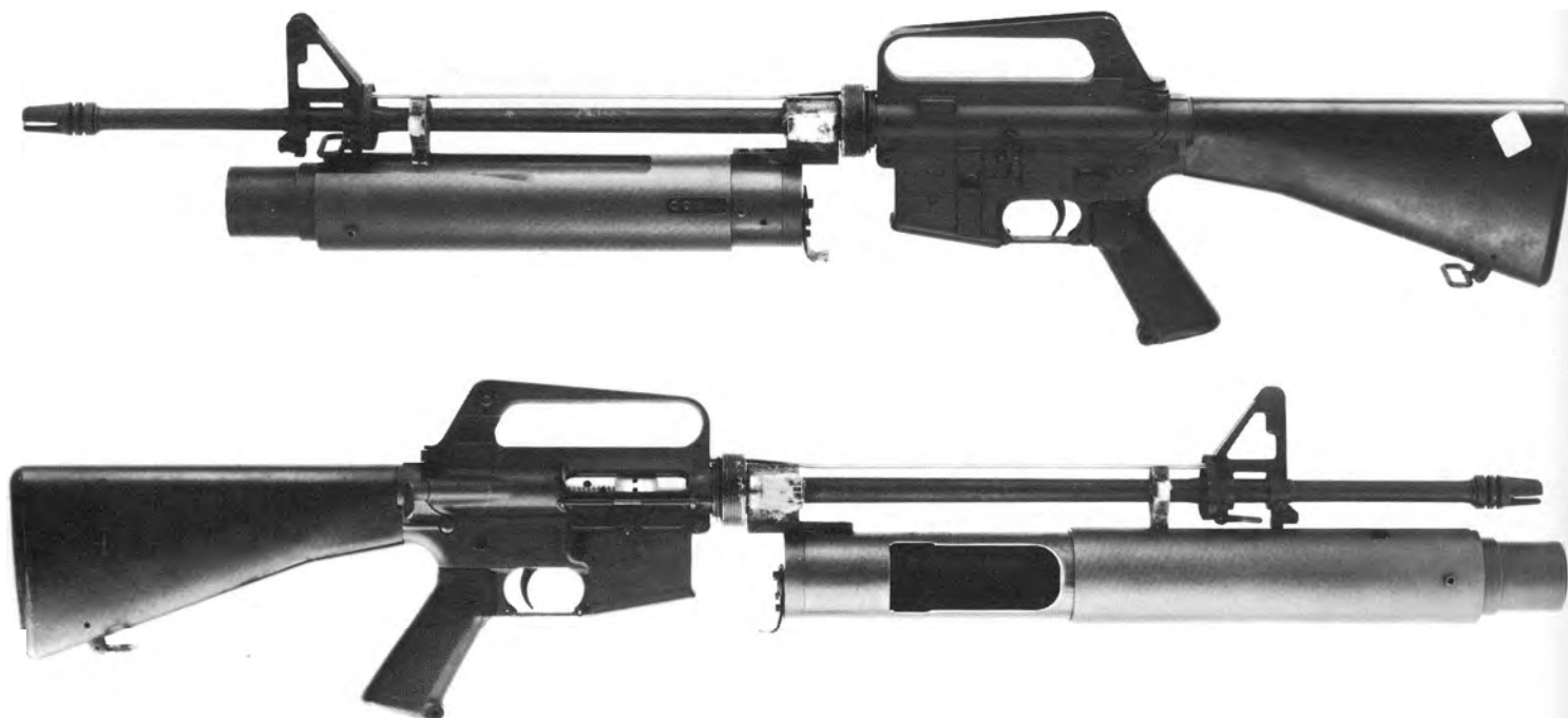
252 Rob Roy's first model of an admirably simple, single-shot 40mm grenade launcher attachment for the AR-15. It was not adopted.
