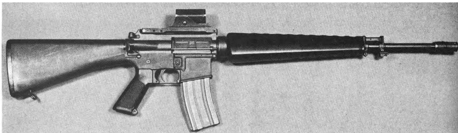
304. An example of blending the fruits of two programs together in the search for enhanced hit probability (Ph). Here a reflex collimator sight (RCS) is mounted on a modified M16A1, rebarreled to fire the "full bore" Frankford Arsenal 4.32x45mm (.17 caliber) "micro-bullet" cartridge
