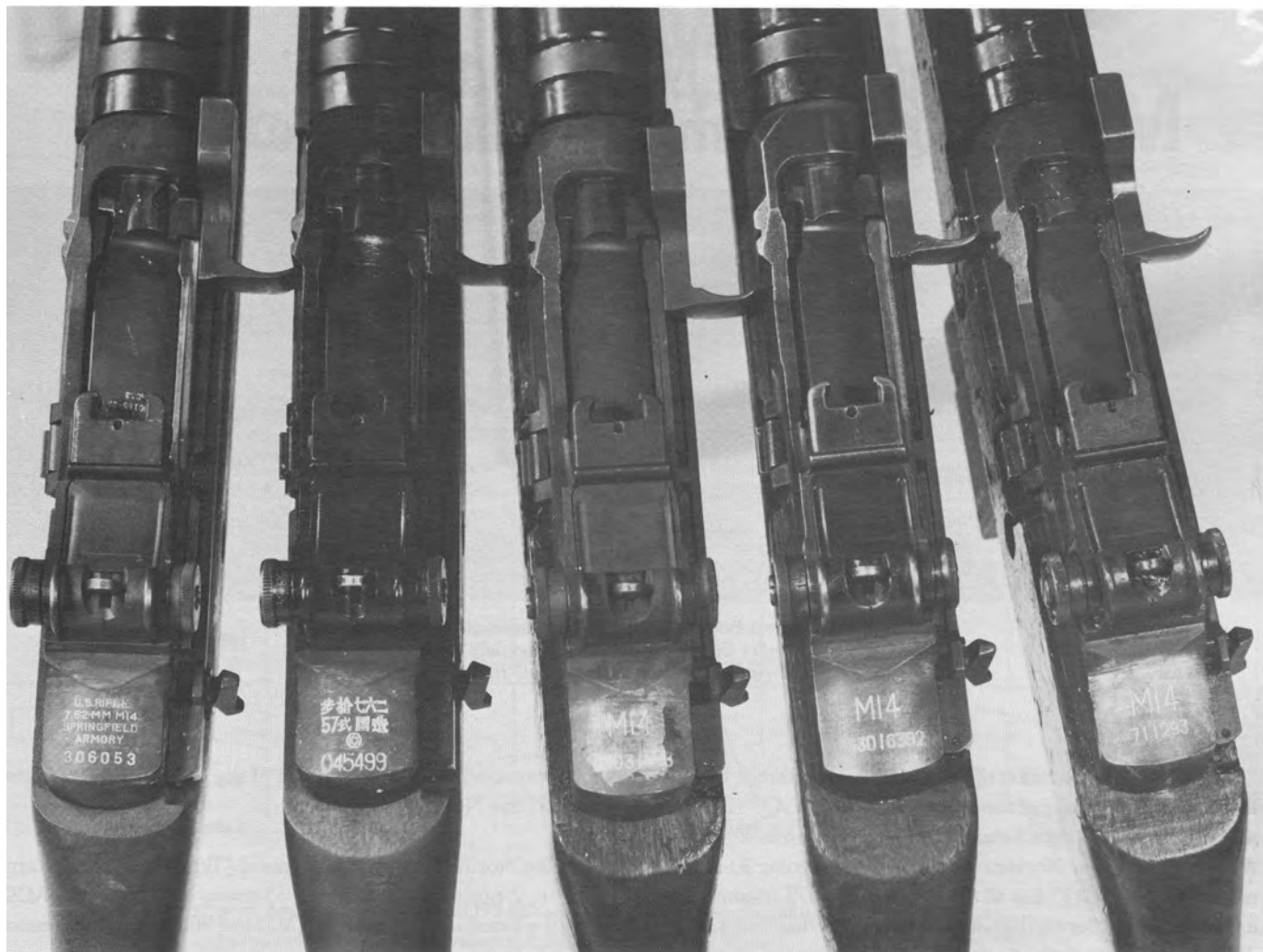
346. Closeup of receiver markings on some typical M14 rifles. From left: 1. genuine US M14, manufactured as part of Springfield Armory's third order for 70,500 rifles, dated March, 1961 (US Rifle M14); 2. Republic of China Type 57
