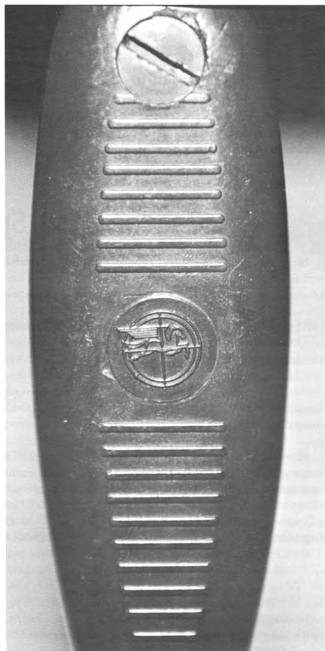
95. Brown molded rubber buttplate (mod. no. 8), the same on both weapons. No drainage hole in screw.
