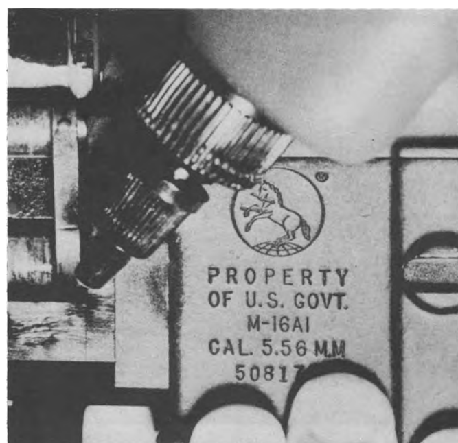
328. Right side view of cross-bolt selector in GL mode.
