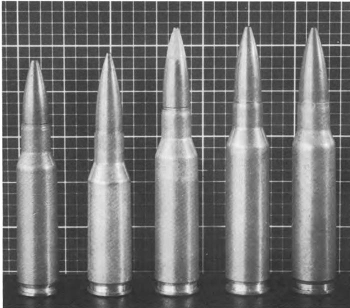
4. Actual-size compendium of UK cartridge development, 1948-1953. From left: 1. the short-lived .270 (7x46mm) early Kynoch manufacture, unheadstamped; 2. the UK trials .280/30 (7x43mm) with base compatible with the US "T65", resurrected in 1970 for UK trials and headstamped RG 701Z; 3. the UK 7x49mm "High Velocity", headstamped RG 52 7m/m H.V.; 4. the joint UK/Belgian/Canadian 7mm "Compromise" (7x51mm), headstamped DAC 52; 5. an early forerunner of the 7.62x51mm NATO, headstamped FN 52. Editor's collection
