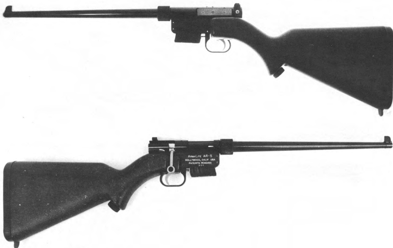
23. Left and right side views of the .22 Hornet caliber ArmaLite AR-5 survival rifle, called by the Air Force the MA-1. The tip of the stainless steel barrel liner is just visible at the muzzle of the aluminum barrel jacket. With the exception
