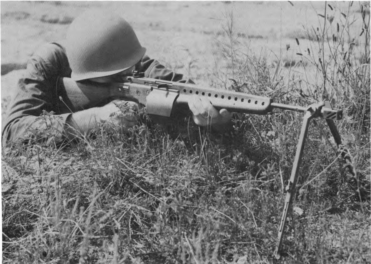
155. The AAI Corporation's first-generation SPIW, chambered for the 5.6x53mm AAI XM110 flechette round (muzzle velocity 4,820 fps; chamber pressure 59,000 psi). This early 5-lb. (point-target version only) AAI SPIW fired 2,400 rpm three-round bursts from a 60-round drum magazine.
