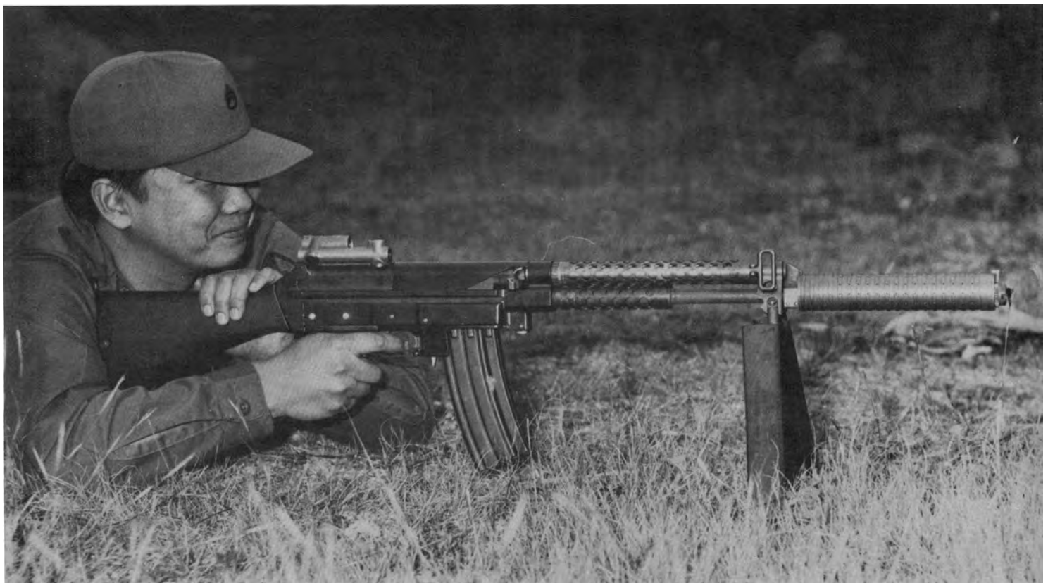
322. US Army Armament Research & Development Command (ARRADCOM) trial of the improved ARES FARC-3, fitted with a metal Stoner 63A magazine. Compare with fig. 321: note how the operating rod handle cams the spring-loaded dust cover open with each shot.
