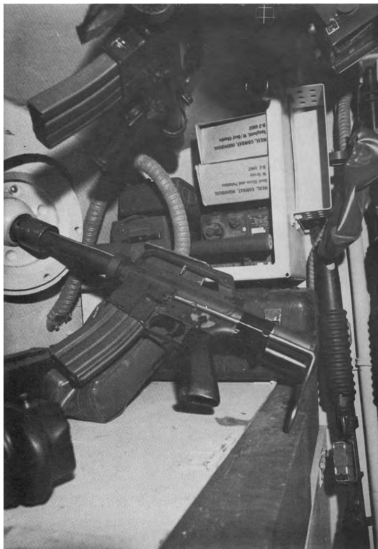
383. A look inside the Bradley IFV, showing an M231 installed in ball-mounted firing port hole, and another in reserve (above). Photo courtesy Bob Faris
