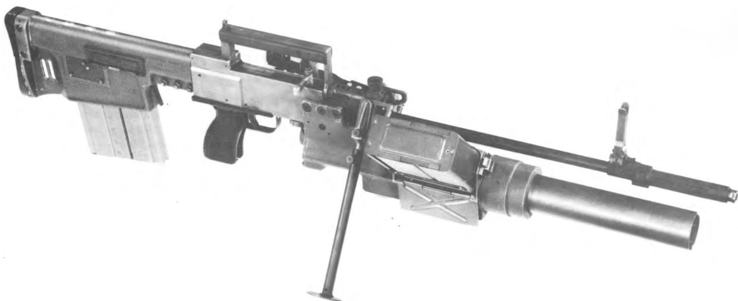
154. Springfield Armory (14.5-lb.) first-generation SPIW. In the words of its designer, the adamant requirement for a 10-lb. weapon carrying 60 point-target flechettes plus three 40mm grenades made the SPIW "the
