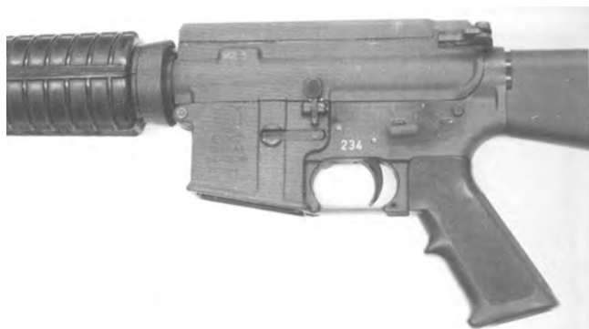
396 A Colt trials model 715 rifle, modified in Canada for low-scope mounting. Canada initially tested a number of sight-enhancement devices for its new 5.56mm weapons which did not require weapon modification. These included standard Colt/Realist 3- and 4-power telescopes; a 1-power, battery-powered, front-sight-mounted holographic dot projector (the "H.R.S.100"); the "Hiteye 1500", a 1.5-power, ring-reticle telescopic sight, also mounted in the carrying handle; and tritium-filled iron sights. A later Diemaco "enhancement" program examined a number of sighting systems fitted to this Canadian-designed handle-less upper receiver (fig. 397).
