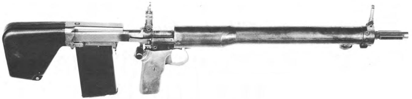
21. John Garand's misunderstood T31, two unfinished handbuilt prototypes of which constituted his final project for Springfield Armory. The magazine
