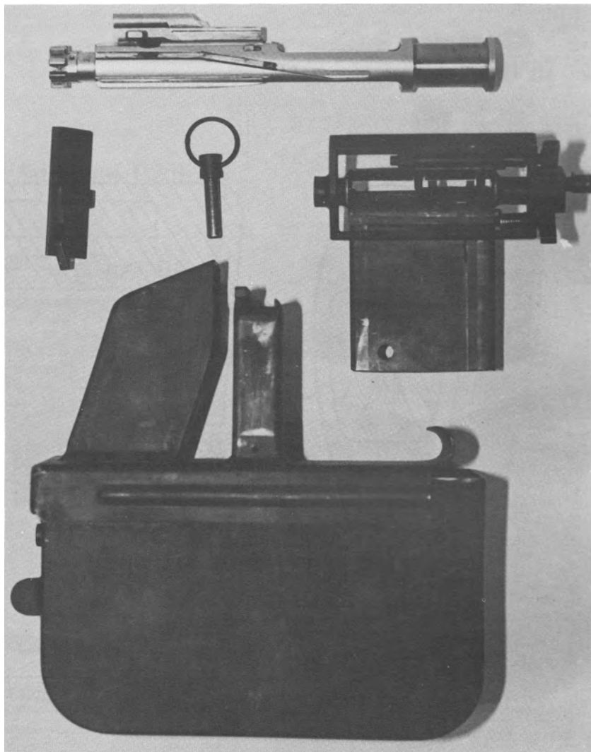
182. Components of the Colt belt-feed system used in the M2 HBAR. Above: bolt assembly (note the longitudinal beltfeed actuating cam slot and lightened rear diameter of carrier). Center, from left: beltfeed actuator; magazine box demounting pin (secures center "dummy magazine" mounting projection of magazine box, below, to beltfeed mechanism); belt feed mechanism, installed down through magazine well of specially modified upper (fig. 181) and lower (fig. 176) receivers. Protrudes below magazine well to accept magazine box and (note hole) demounting pin.
