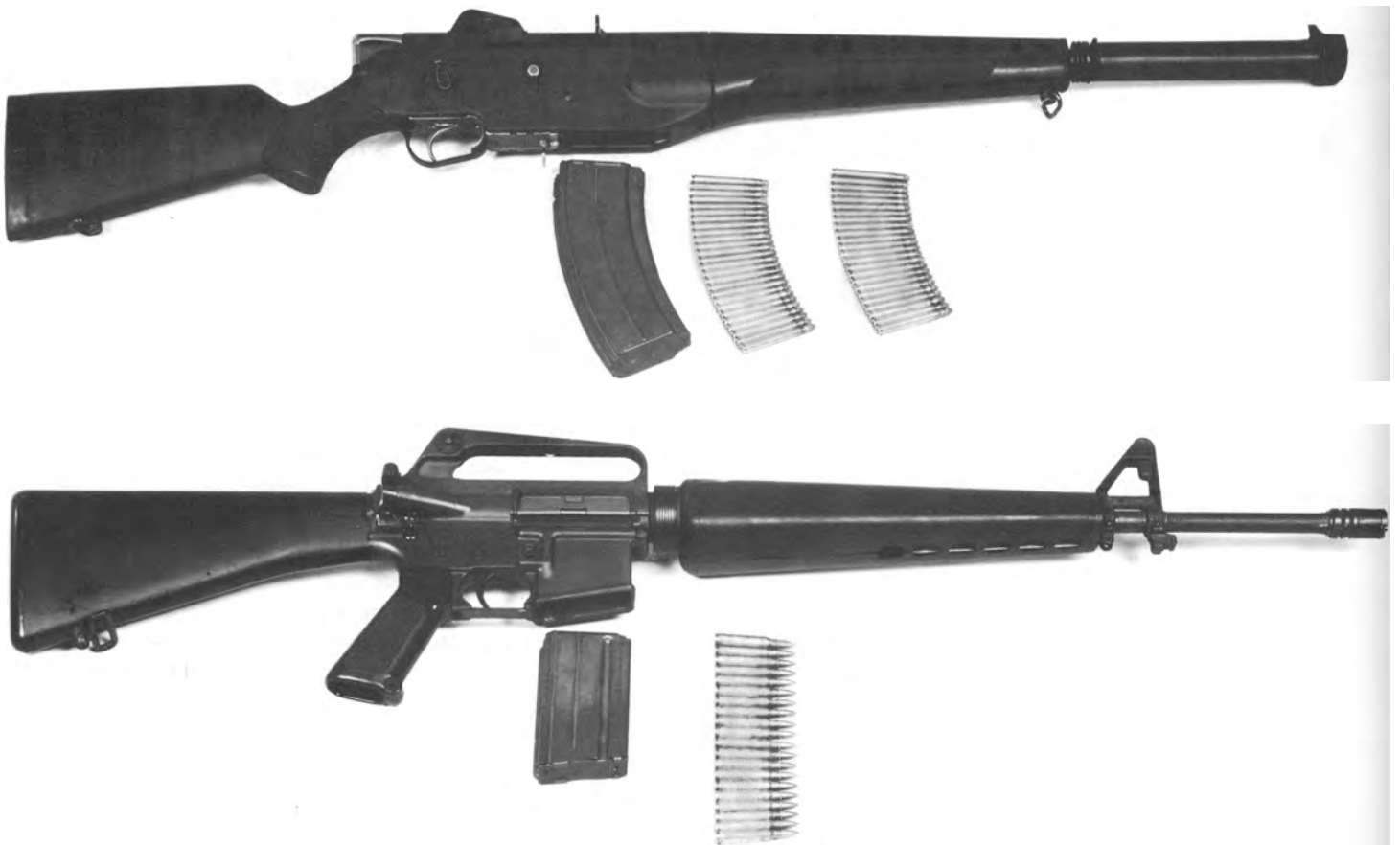
294. Above: the AAIXM19 serial flechette rifle (SFR), with new 50-round box magazine. Caliber 5.6x57mm XM645 (fig. 218 no. 3). This 1969 contract was the first award of an official "XM" number to a SPIW candidate.
