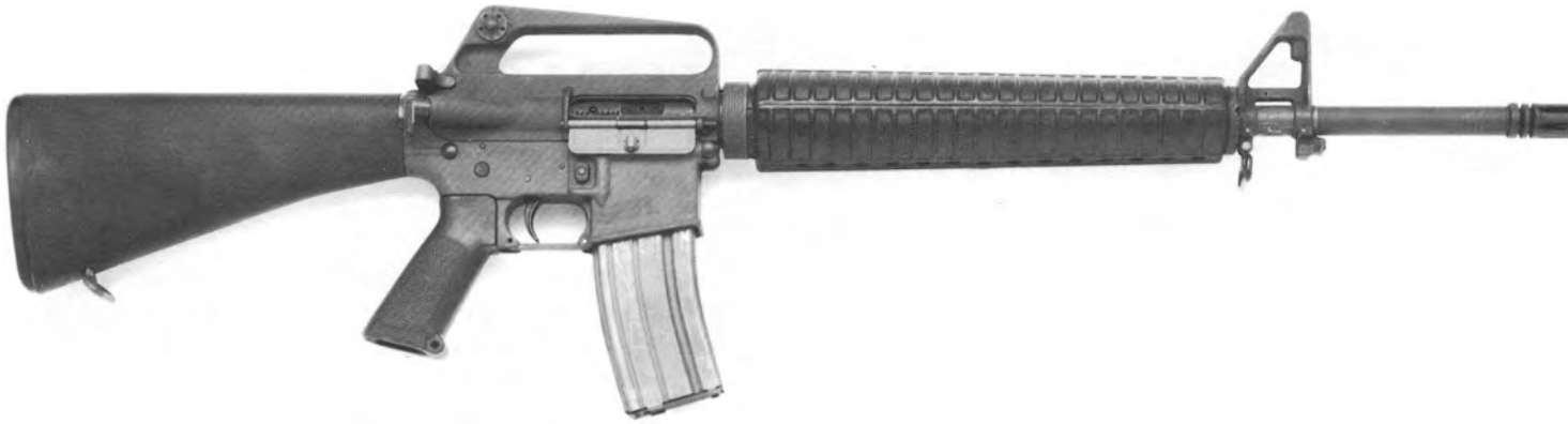
369. Right side view of early M16A1E1 rifle. Not yet fitted with the spent case deflector "lump" on the receiver (fig. 371).
