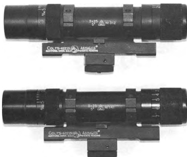
118. Left side view of two Delft Optics AR-10-type 3x25-power telescopes (fig. 58) adapted as the "TTL-80" the first AR-15 scope sight. Note the different types of finish; serial no. 312 (above, dull); and serial no. 141 (below, bright anodized) in early Colt-made mount (part no. 62215).
