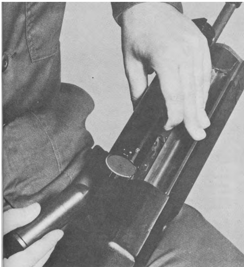
327. Loading the four-shot HEL 30mm GL. Two rounds were first inserted in the (2-round) forward portion of the magazine, shown. Closing and latching the magazine automatically pushed one grenade back into the rear (1-round) magazine. Pushing the charging lever (of the blow-forward launcher) forward and allowing it to snap back chambered the rear round, and replaced it in the rear magazine with the round remaining in the forward magazine. The empty forward magazine was then recharged with two more rounds.
