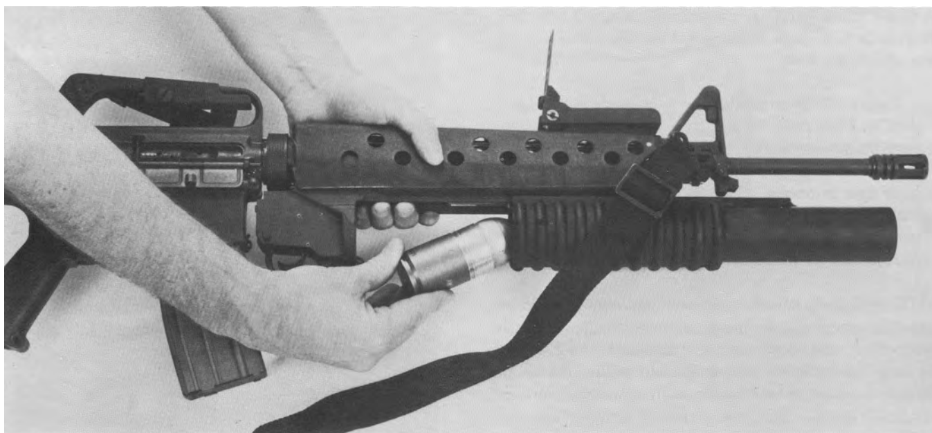
252. Right side view of the M16A1/M203 combination, showing the barrel forward and a grenade being inserted. Extraction takes place on the forward
