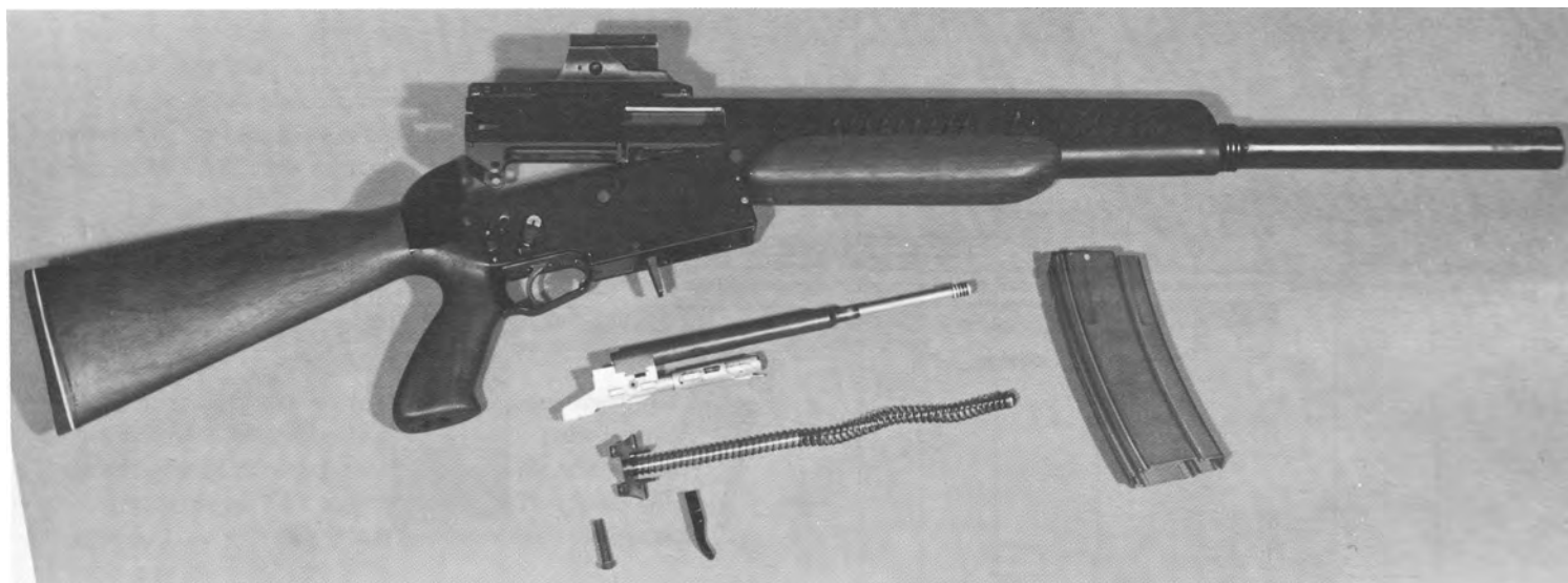
311. The partially-stripped, 4.32mm prototype of the AAI serial bullet rifle (SBR), first unveiled at a Fort Benning conference in May of 1977. The 10-lb., clip-fed AAI SBR featured a unique, two-mode firing system (semi auto and 3-round burst only) wherein the firing pin was hammer-actuated
