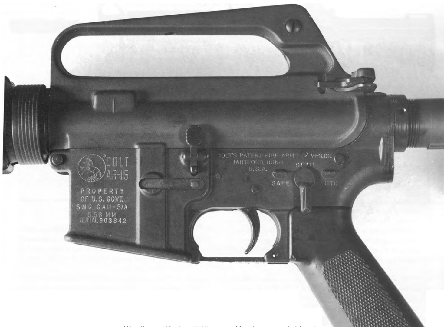
231. Closeup of the later USAF version of the telescoping-stock "shortie": the bolt-closerless XM177 (Colt model 649). Barrel length: 14" overall, including suppressor. Note the Air Force marking "GAU", standing for "Gun, Automatic".
