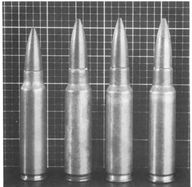
5. The (actual size) US counterpart to fig. 4. From left: the original "Case, Cartridge, Light Rifle" (7.62x47mm) loaded with a double-cannelured M2 ball bullet and headstamped FA 45; the Frankford FA-T1 (7.62x49mm) circa 1948-50, headstamped FA * 48; the FA-T1E1, headstamped FA 49; and the FA-T1E3 (7.62x51mm, the forerunner of the 7.62 NATO), headstamped FA 50. Editor's collection
