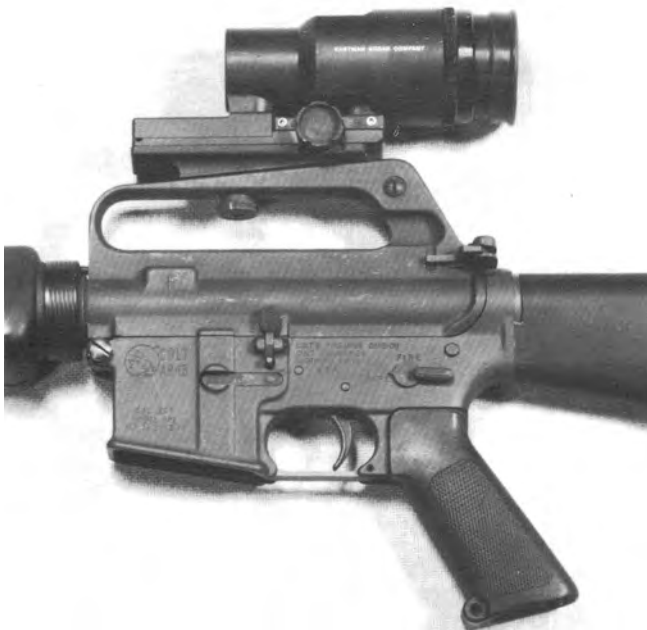
379. Closeups of a civilian AR-15 (model SP1), fitted with experimental Kodak 3.5x Optical Sight.
