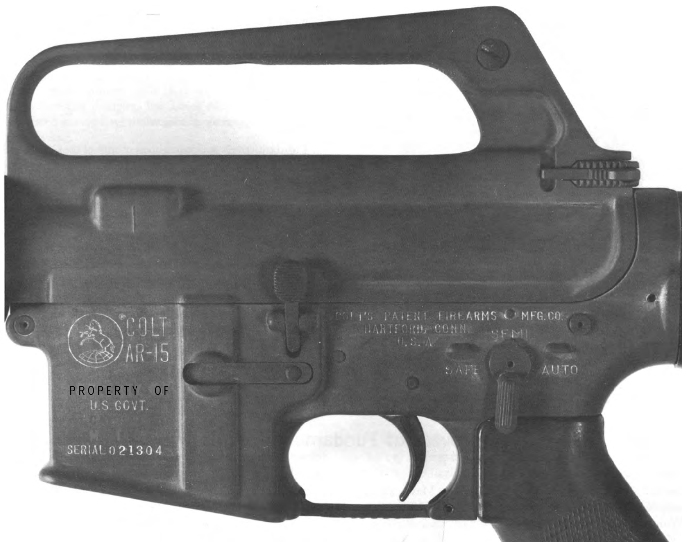
140. Closeup of the receiver markings on a Colt AR-15 model (6)02, the precursor to the XM16E1, serial no. 021304. Black-impregnated furniture,
