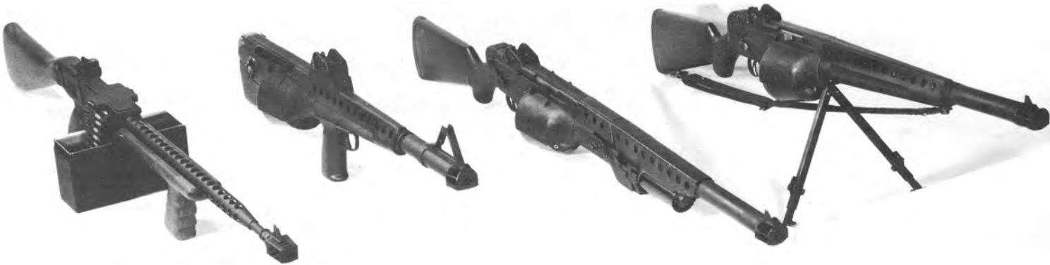
216. The AAI "SPIW Weapons Family" circa early 1966. From left: prototype belt fed LMG (note early square-section muzzle brake); prototype "bullpup" SPIW Carbine; second-generation SPIW rifle, caliber 5.6mm
