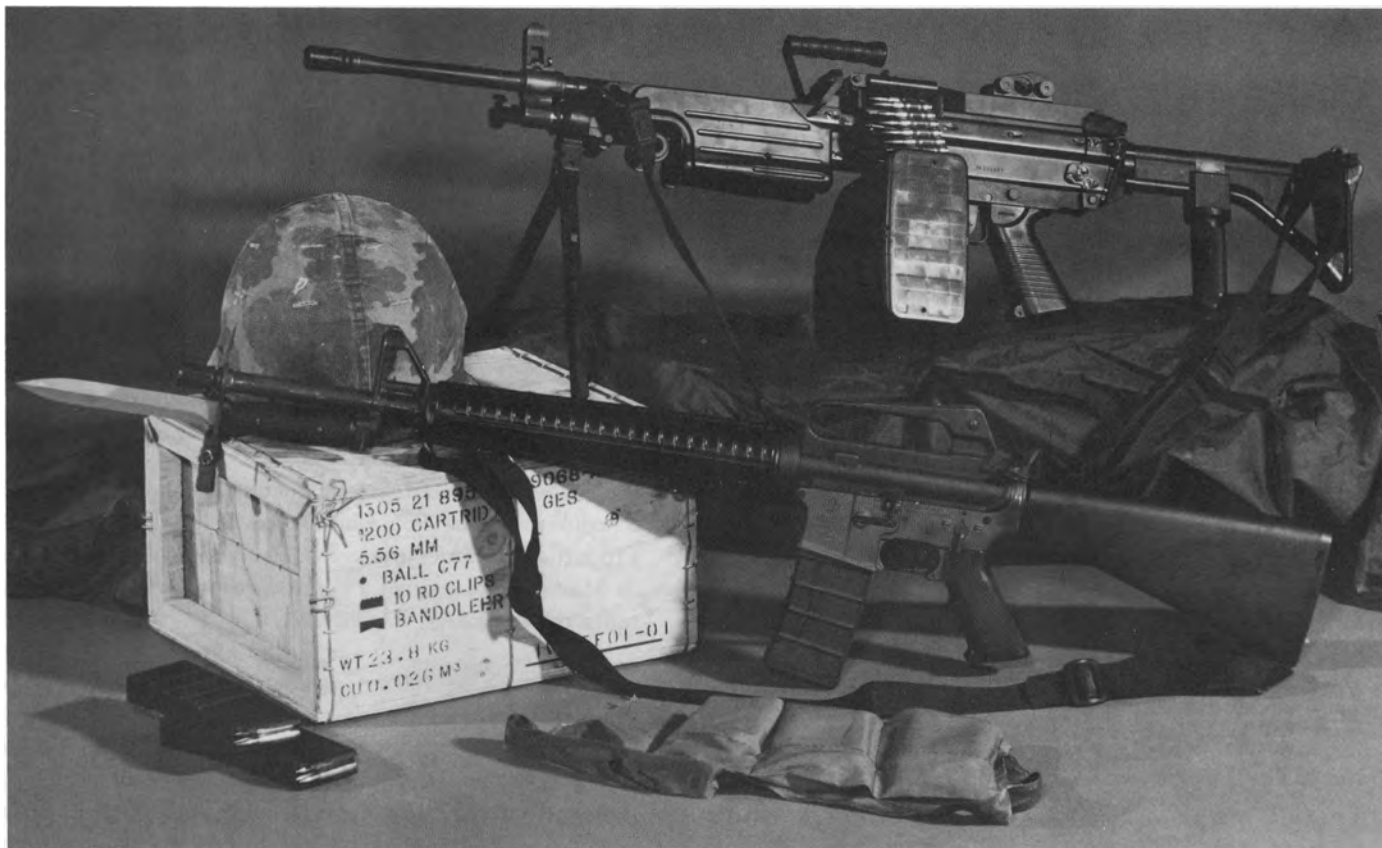
392. Canadian Forces 5.56mm C7 rifle and C9 (FN Minimi) light machine gun, with equipment. Type 3 receiver markings (fig. 389). Note the ammunition supply packaging: 30-round Canadian-made nylon magazines are charged from
