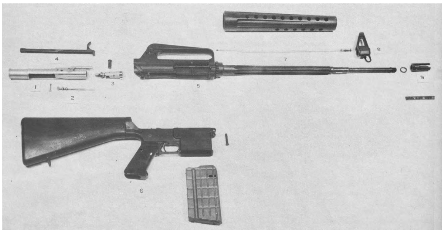
52. Another Detroit Arsenal "Tech n'Tell" photo, showing an exploded view of the early A-1 AR-10 "Sudan" model, right side. Note the fluted steel barrel.
