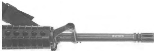
440. Markings on the proposed C10 .22LR training rifle from Diemaco, Inc. : 22LR TW 1/16.
