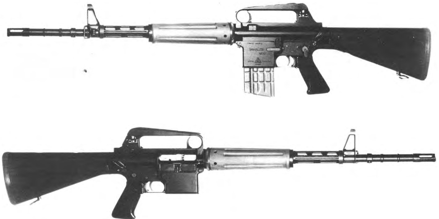
54. Left and right side views of the Dutch second, or "transitional" model AR-10, serial no. 003837. Note the redesigned grenade-launcher/barrel and composite wood-and-stamped-metal forend. The "transitional" model was fitted with a non-fluted barrel, an improved trigger group with an additional trigger spring, a reworked selector lever with SAFE now forward, and a re-
