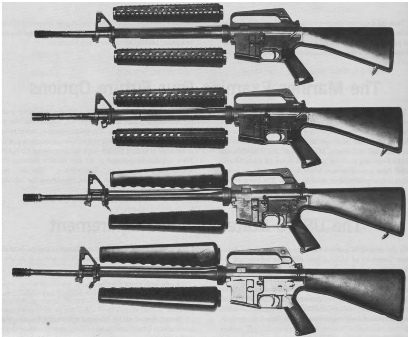
365. From the August, 1980 1-in-12 heavy-barrel trials conducted at the Naval Surface Weapons Center, Dahlgren, Virginia. Top two rifles (serial nos. 4833958 and 4833992) are fitted with heavy barrels (note the difference
