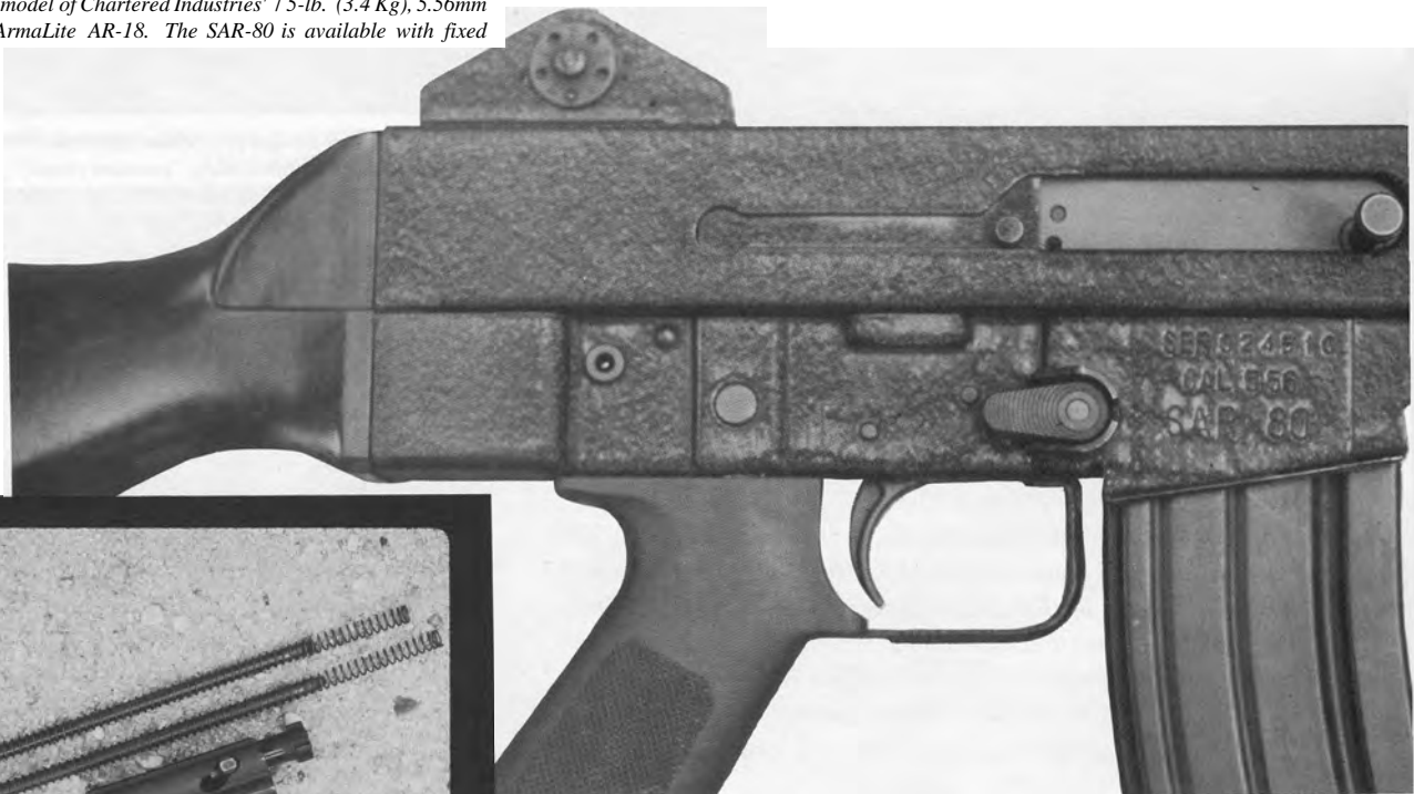
337. Closeup of right side of late model (redesigned pistol grip; ambidextrous magazine catch) SAR-80, showing receiver markings.
