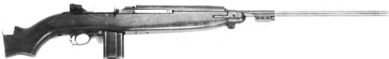
16. Experimental .22 M2 Carbine, serial no. 7548460. Stock cut off at wrist and holes in forestock (ahead of magazine) for mounting in test fixture; steel tube attached to operating slide to facilitate measurement of com-
