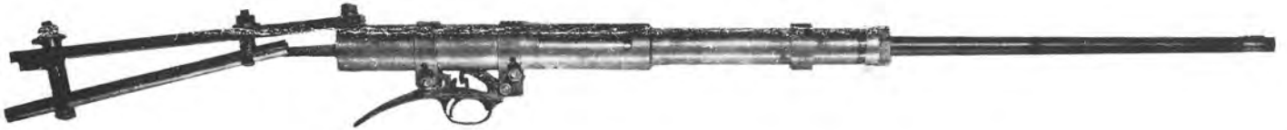
27. Melvin M. Johnson Jr.'s first working model of his short recoil action, hand-built in a shop in Boston in 1936. Photo courtesy Bob Miller
