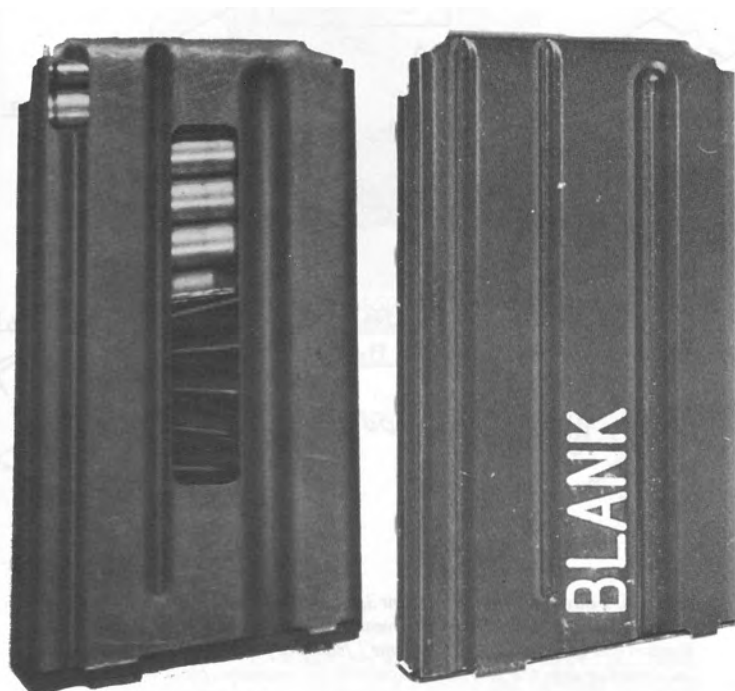
411. Magazine for instructional cutaway rifle, showing positioning and feeding of cartridges. Photo courtesy Steve Kemp
