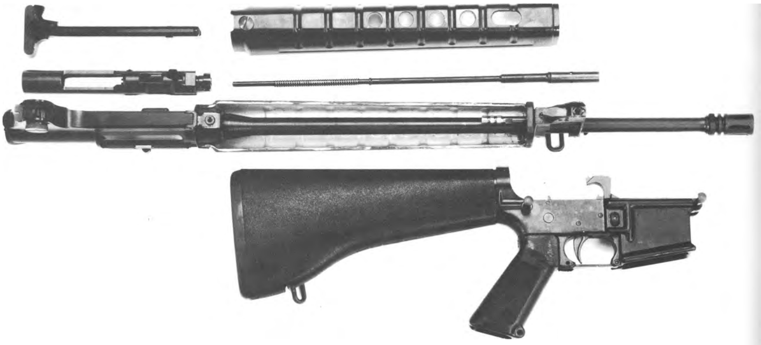
345. Partially-stripped view of the 5.56mm Taiwanese T65. Note from top: M16 charging handle, new upper handguard; AR-18-type gas piston assembly and M16 bolt assembly sans carrier key; M16-type (bolt closerless) receiver
