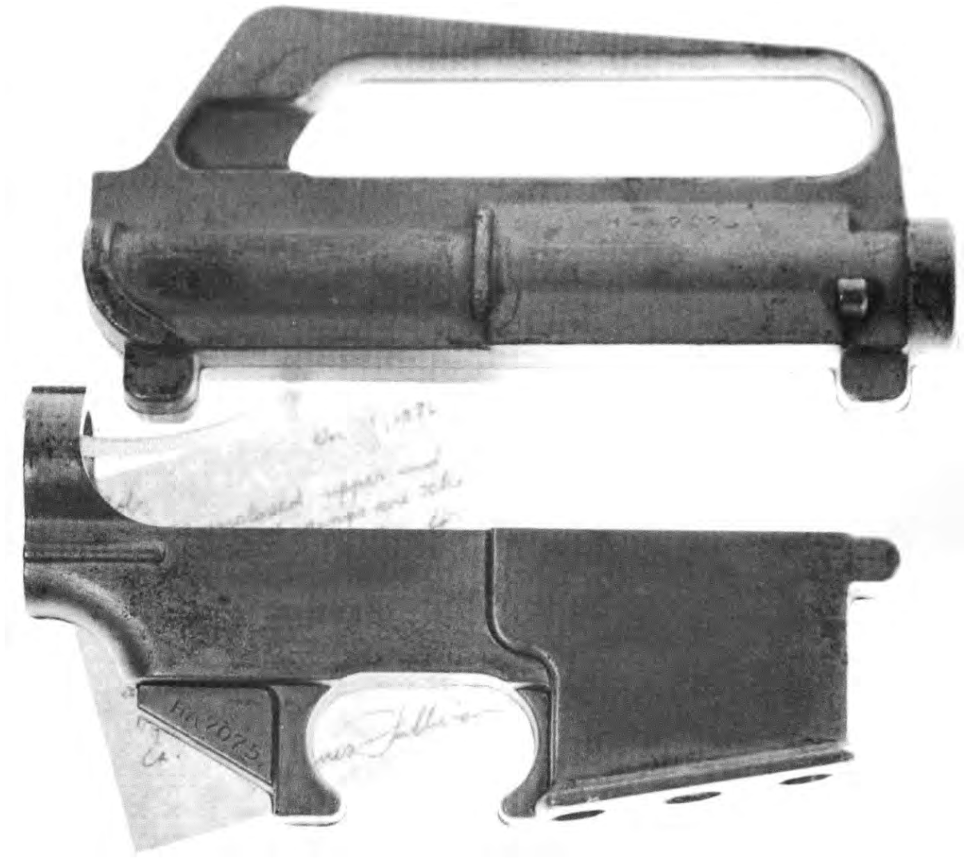
77. Unmachined examples of the earliest production run of AR-15 receiver forgings. The note underneath, from AR-15 designer L. James Sullivan to collector Bob Miller, reads as follows: "...The enclosed upper and lower receiver forgings
