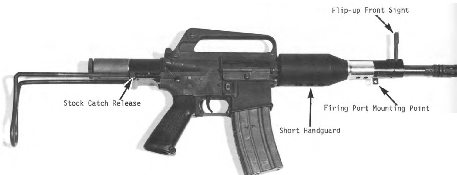
381. A later prototype of the XM231 Firing Port weapon. Note the flip-up front sight; the short handguard; and the telescoping stock: all attempts to
