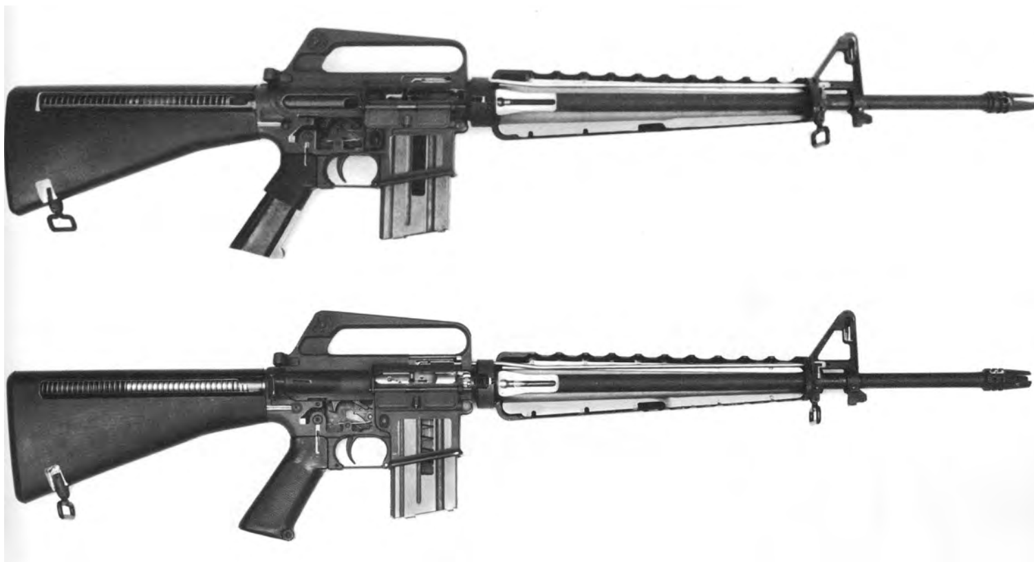
150. Above: a Colt factory "cutaway" of an AR-15 (XM16E1) model 02. Compare with fig. 130. Bob Miller collection, photo by Roy Arnold Below: a later (XM16E1) cutaway with bolt closure device.
