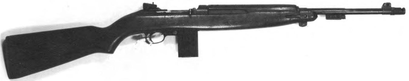
13. The .22 Gustafson Carbine, right side view. Made from a standard M2 Carbine manufactured by the Inland Division of General Motors Corporation of Dayton, Ohio, serial no. 7125359. Regular 15-round magazine holds only 10
