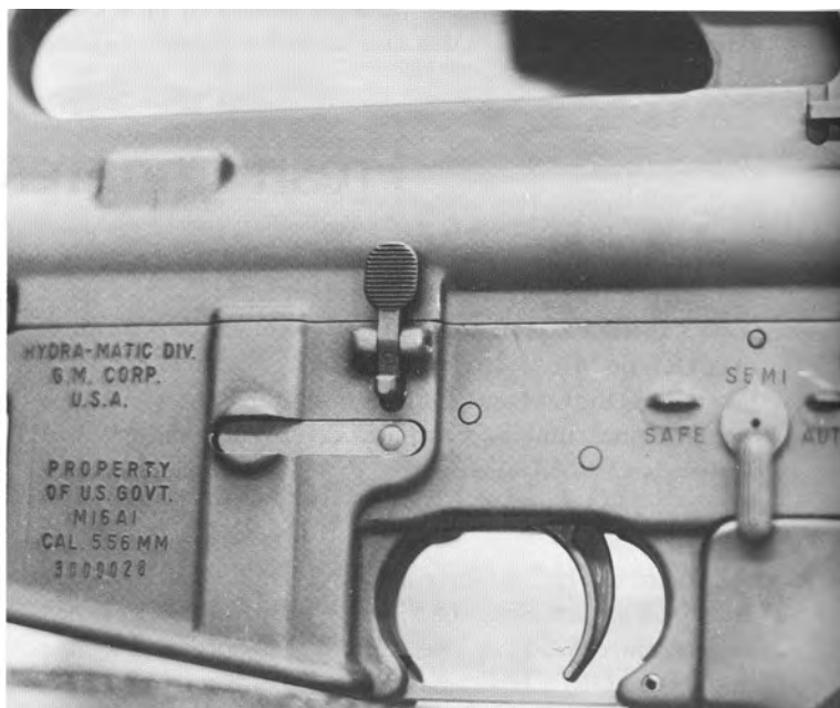
280. Closeup of receiver markings on a typical M16A1 as manufactured by the Hydramatic Division of General Motors Corporation. Note serial no. (28th rifle in GM's assigned serial no. range, which began at no. 3,000,000).
