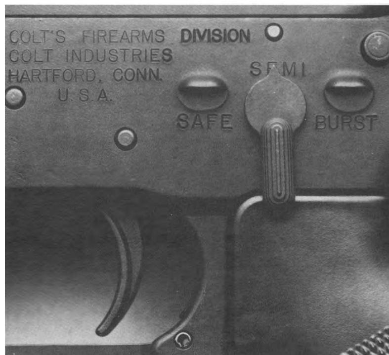
372. Closeup of receiver markings on early production version of the M16A2 rifle (8-million-series serial nos.) This is no. 8000031. Note the new, finger-grooved pistol grip.
