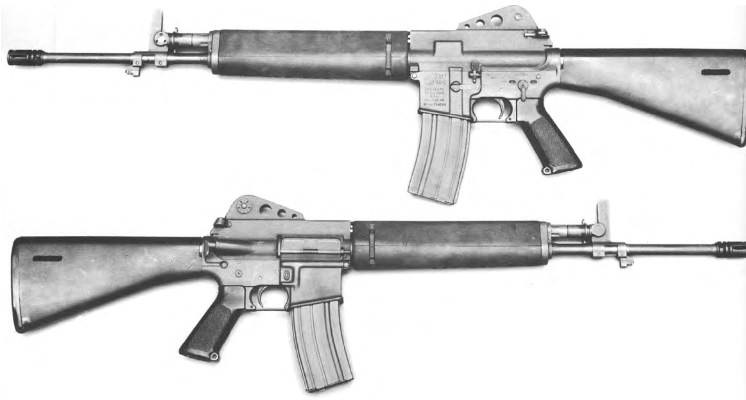
275. Left and right side views of a later prototype Colt model 703. Note (above) the adjustable, three-position gas regulator, much like that of the Stoner XM22E1
