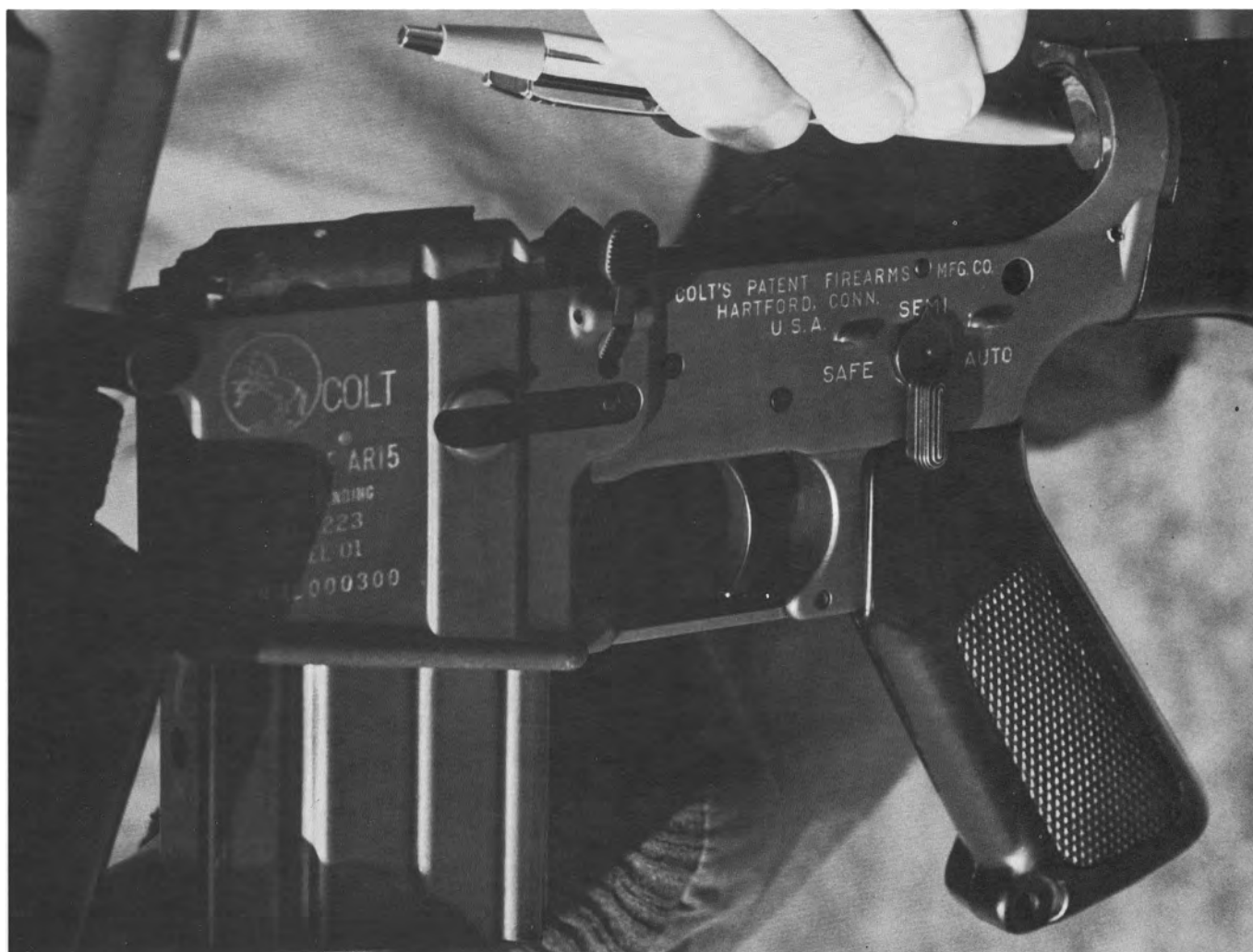
111. From Colt's first run of AR-15s: pointing out the "recoil spring guide" on Model 01 serial no. 000300.
