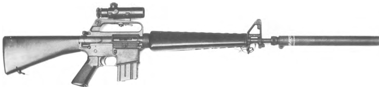
265. Right side view of a Colt M16 rifle fitted with the MAW-A1, the 5.56mm version of the Sionics noise and flash suppressor, and the Colt/Realist 3x telescope sight. Note the remains of the milled-off bolt closure device housing on the rifle's receiver. This rifle was probably made during the "standoff"
