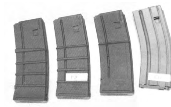
421. An early GAPCO nylon 30-round magazine. Numerous styles and models of all-plastic magazines have been developed for the M16, the most successful being the Canadian pattern (figs. 392 and 422).
