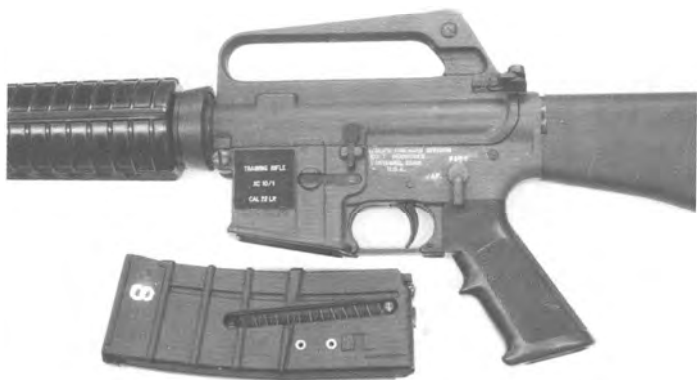
440. Markings on the proposed C10 .22LR training rifle from Diemaco, Inc. : 22LR TW 1/16.
