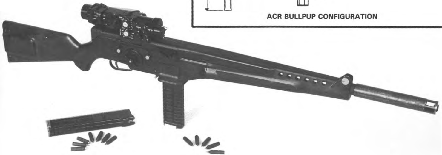
332. The AAI ACR, right side view, showing a few of the "heavy-bullet" 5.56mm loads (left) and some 4.32mm "sabot-bullet" rounds (right). The ACR drew heavily on experience gained during the XM19 and XM70
