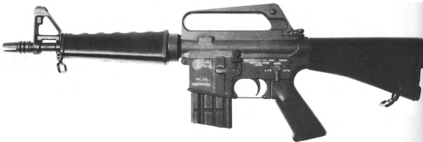
185. Another one-off, toolroom model of the CAR-15 submachine gun, made from AR-15 serial no. 014864, featuring the plain (model 02) flash suppressor on a 10" barrel. No bayonet lug; export markings; early steel "waffle" magazine; standard pistol grip and extendable buttstock.
