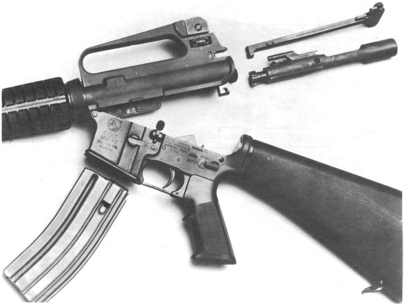
372. Closeup of receiver markings on early production version of the M16A2 rifle (8-million-series serial nos.) This is no. 8000031. Note the new, finger-grooved pistol grip.
