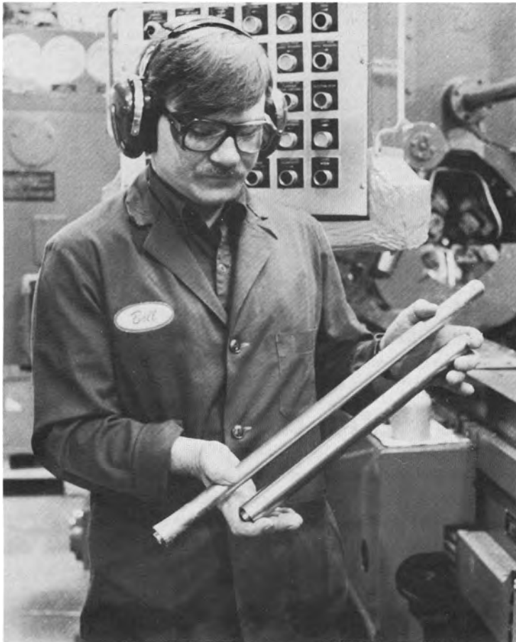
391. C7 and C8 barrels are made on this government-supplied, state-of-the-art hammer forge from GFM of Austria, the only one of its kind in Canada. This powerful machine takes a carefully honed, smoothbore "blank" (below) and exerts tons of pressure on the outside surface in a continuous and extremely rapid multi-hammering process, drawing the blank out roughly one-and-a-half times its original length and cold-forging it down around a hardened mandrel. The mandrel, about six inches long, is perfectly formed in the shape of the chamber, lead and the first few inches of rifling. Concentrating initially on the rifling section, the blank is slowly rotated as it is hammered, the mandrel being simultaneously withdrawn until the end of the blank approaches, whereupon the mandrel stops while the hammers continue, thus cold-forming the complete bore and chamber configuration all in one pass.
