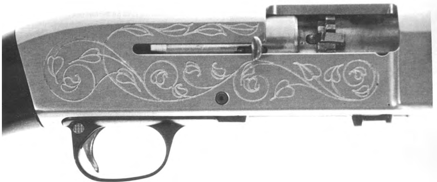
25. Closeup of the receiver of the ArmaLite AR-17 "golden gun" showing the rotary lugs on the bolt, which lock into the steel extension/liner of the barrel. The AR-17 Junctions on the short-recoil principle.
