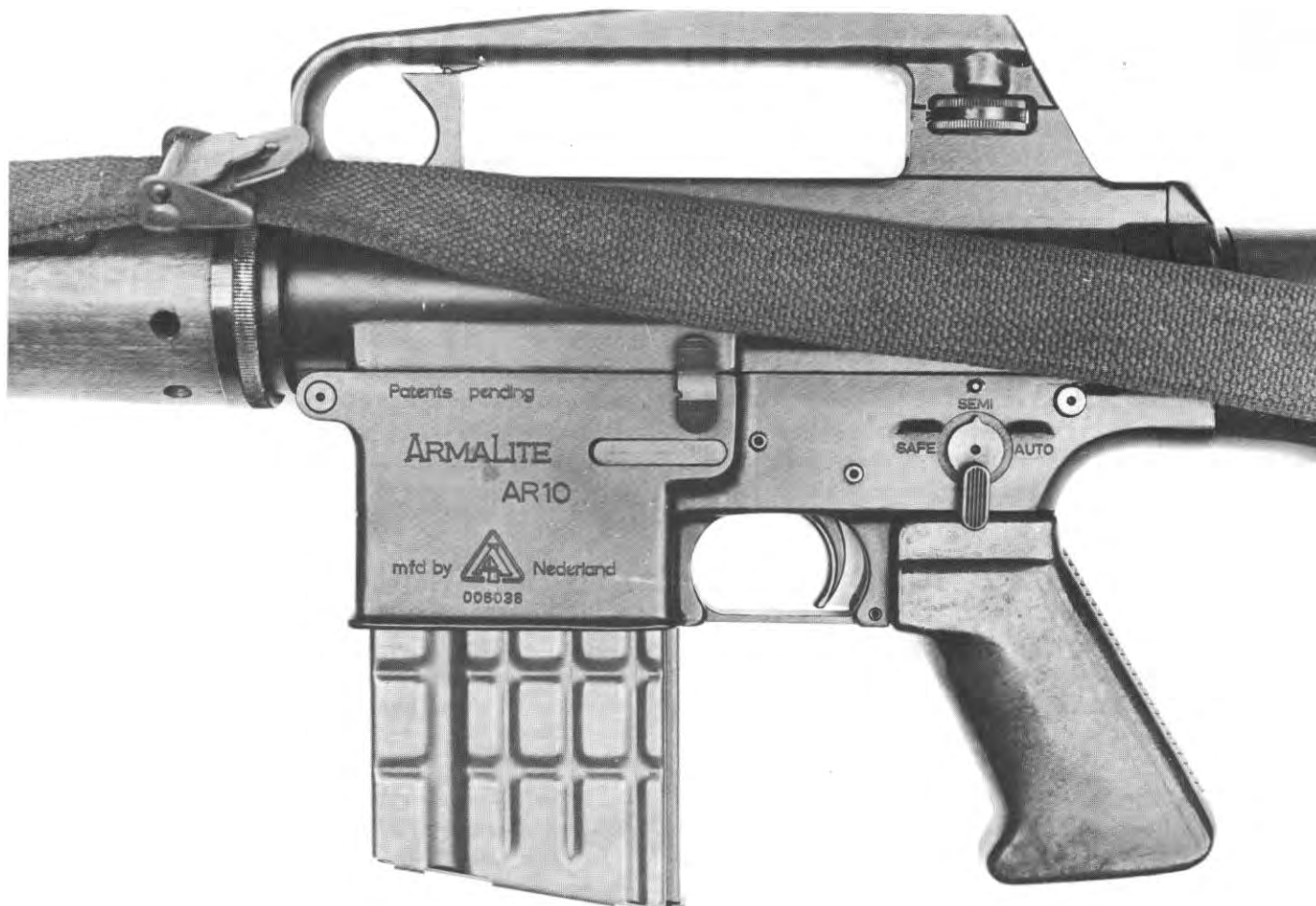
66. The final model of the Artilerie-Inrichtingen AR-10, produced for the South African NATO-caliber rifle trials in 1960 and later adopted by Portugal. Serial 006038. The "NATO" or Portuguese model AR-10 features the "transitional" wood half-handguard with its stamped-metal liner protruding up to the gas
