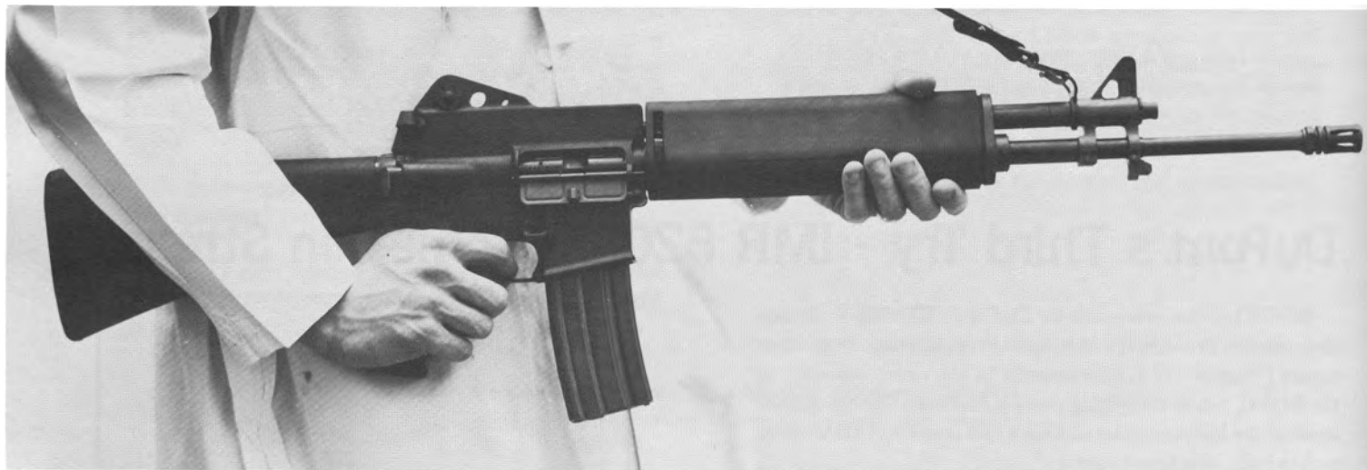
274. The first prototype of Colt's gas piston-operated "model 703", built from a new upper receiver and gas piston system on a standard M16A1 lower receiver. Shown ready to fire in the sling-mounted, waist-level position. Note the full-curved 30-round magazine. (Compare with fig. 275: visible changes in the
