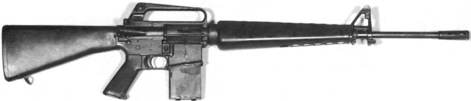
316 A rare photo showing an M16A1 rifle converted to fire 6mm XM732 ammunition (fig. 306 no. 5) in support of the SAW program. Note the flash suppressor from the Rodman SAW, the XM235 (fig. 317) and the receiver and magazine,
