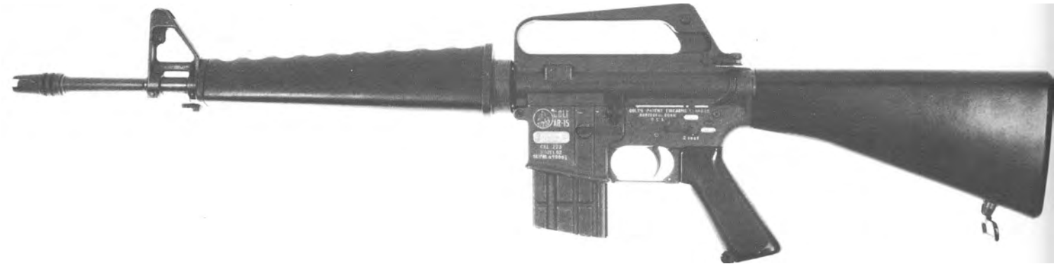
166. Factory prototype CAR-15 Carbine, with a shorter handguard, a 16" barrel and a modified, 4-position selector mechanism. Selector markings for
