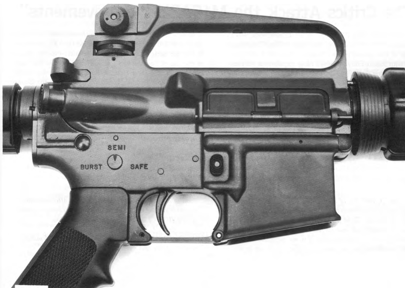
377 Closeup views of both sides of the receiver of a later M16A2 "Commando". Note the selector markings on both sides and the newer, chamfered rear sight windage knob (fig. 375).
