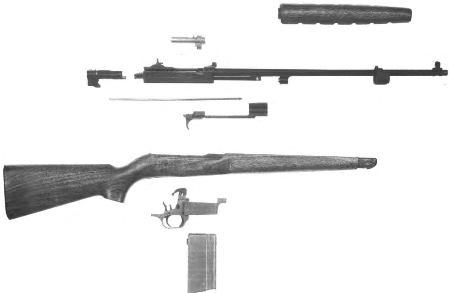
79. Winchester Light Weight Military Rifle serial no. 2, disassembled. The resemblance to the M2 Carbine, especially in the bolt, operating slide and short-stroke gas piston, is unmistakable.
