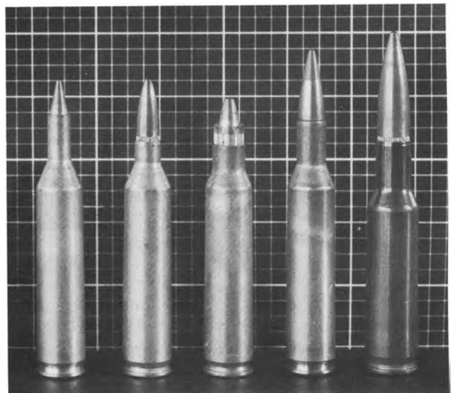
306. Further (actual size) cartridge development. All but no. 5 are based on the standard 5.56mm (M193) cartridge case. From left: 1. one of several types of 3.5mm micro-bullet designs from Fabrique Nationale, headstamped FN 73; 2. Frankford Arsenal 4.32x45.6mm (caliber .17) "full bore" ball, headstamped FA 73; 3. the "saboted .17", which was designed to offer the .17's specialized, lower recoil signature (fig. 294) interchangeably with regular 5.56mm loads in standard M16s, headstamped LC 72; 4. UK 4.85x49mm tracer (red tip), headstamped RG [Radway Green] 77485; 5. the 6x44.5mm XM732, one of several experimental cartridges developed for the SAW program, with olive-green lacquered steel case headstamped FA 73. Author's collection
