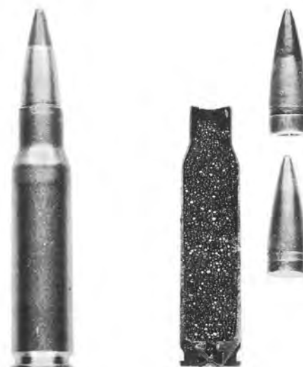
143. Above: the green-tipped 7.62x51mm M198 Duplex round, adopted on May 7, 1964, shown loaded with Olin's WC846 ball powder. Note the dispersion-inducing 9° cant on the base of the lower bullet.
