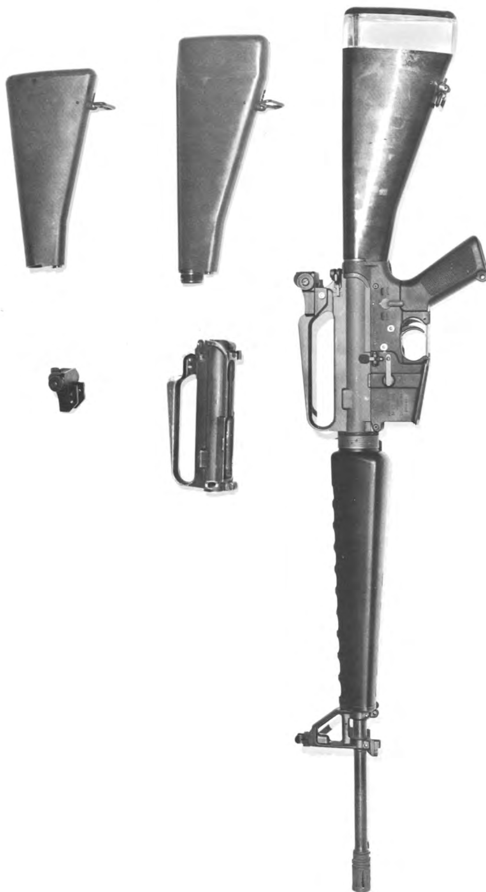
350. The Rock Island Arsenal version of the M16A1 National Match Rifle, showing rifle assembled (below) and altered components (above).
