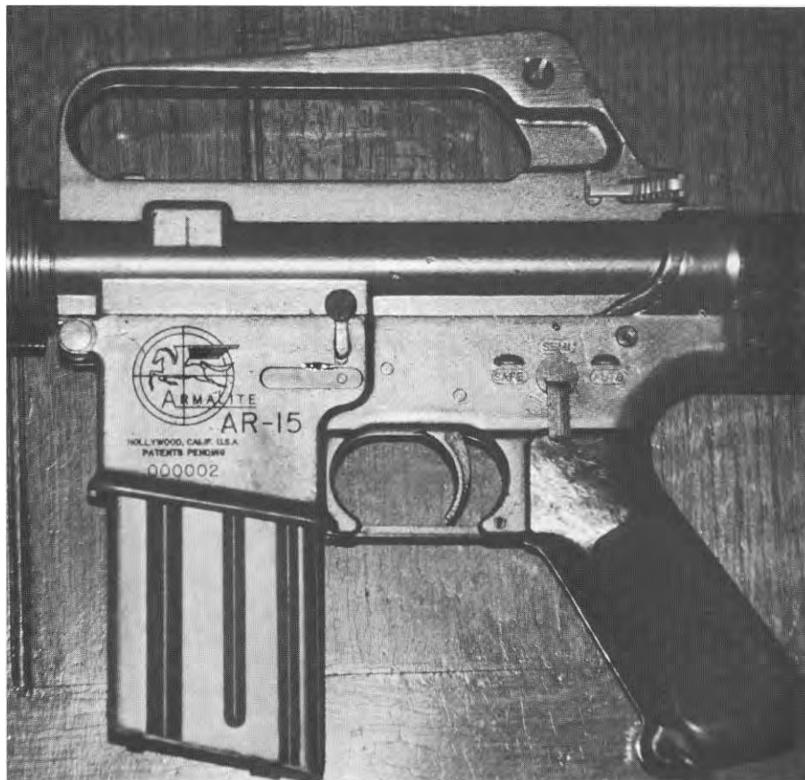
88. A closeup view of the receivers, left side, of the earliest ArmaLite AR-15s. Although serially numbered earlier than no. 000012 (fig. 75), various modifications, such as those recommended after the initial Infantry Board trial in March, 1958 have been made to both weapons. Rifle no. 000002 (above) has an experimental grooved slip ring and hence a two-
