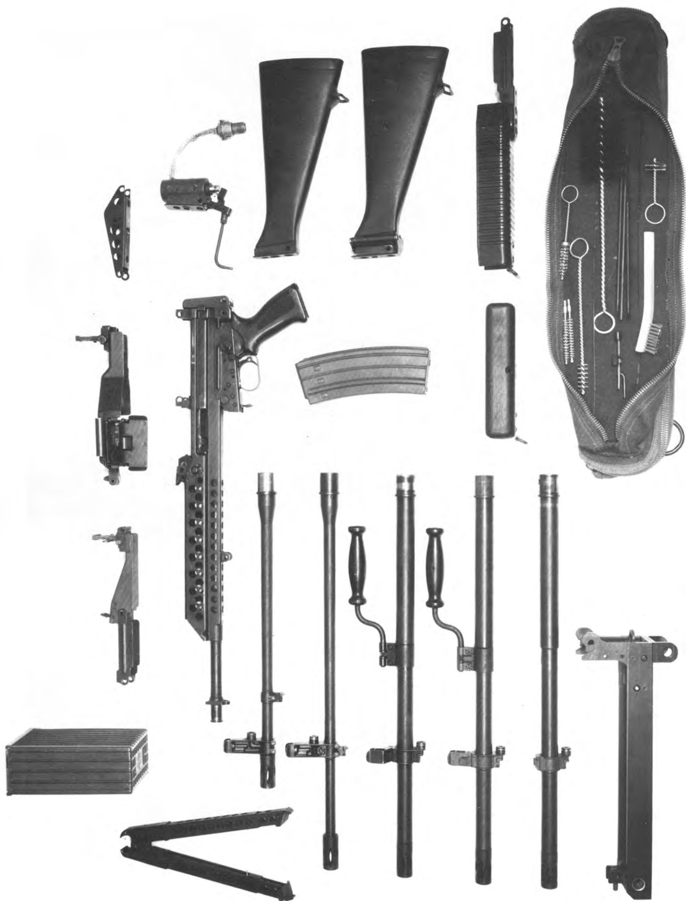
193. The complete 5.56mm Stoner 63 system, as favored for adoption by the US Marine Corps, and tested in the SAWS study. The Stoner system boasted over 80% parts commonality among all its versions.
