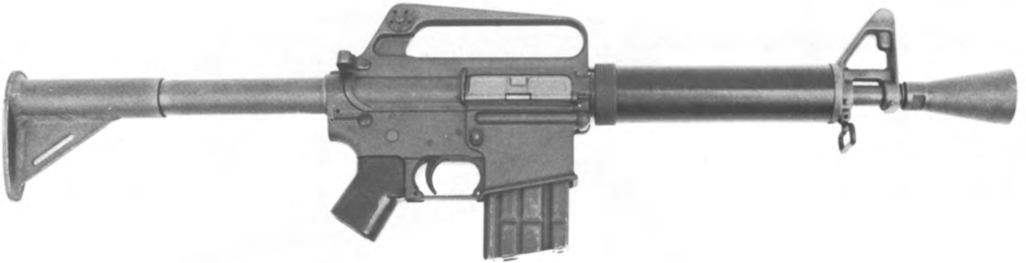
186. Right side view of two CAR-15 survival rifles (Colt model 608). Above: note the unique funnel-type flash hider and distinctive round handguard, the "bobbed" pistol grip and non-adjustable metal stock.
