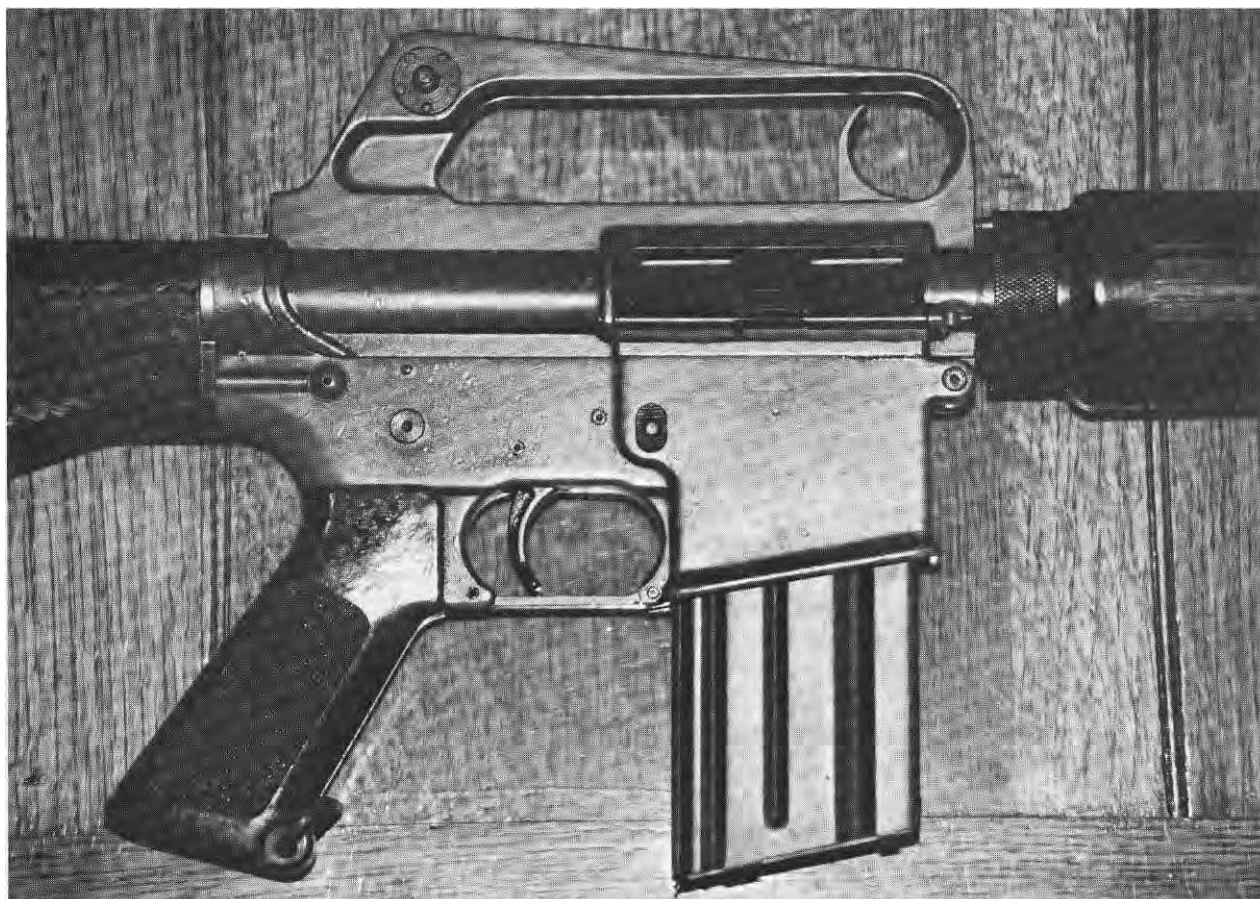
89. Closeup of the two receivers, right side view. No. 000002 (above) with modified charging handle. Both weapons feature woven fiberglass buttstocks, pistol-grip sling swivel, and the original 25-round magazine.
