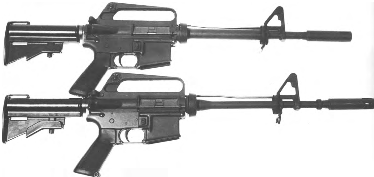
229. Right side view of two more experimentals from the Colt model shop. Above: an M16A1 fitted with an unusual 11" heavy barrel. Below: final 11 1/2" barrel configuration as used on the XM177E2. Bob Miller collection, photo by Roy Arnold
