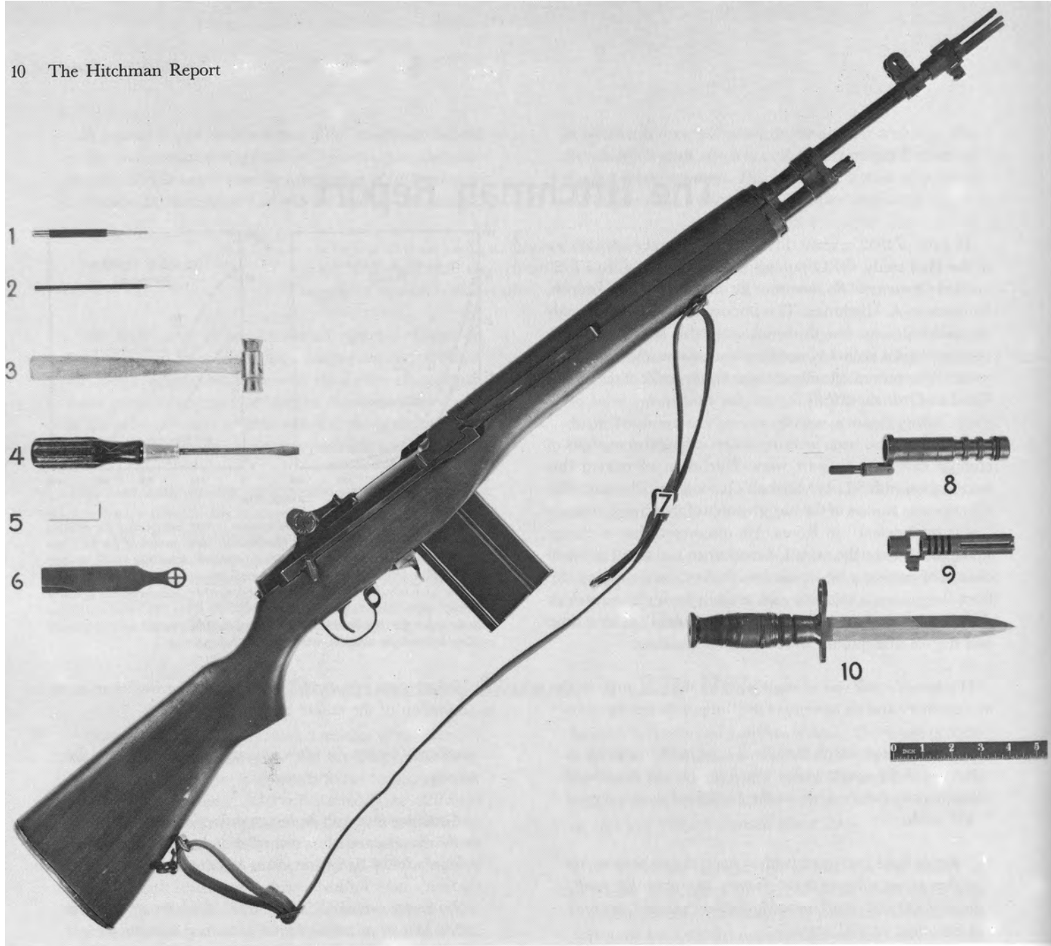
10. An early version of the "Rifle, Lightweight, Cal. .30, T44", built at Springfield Armory on a lengthened M1 rifle receiver. The T44 succeeded the T25/T47 as Col. Studler's US contender in the 1952 international
