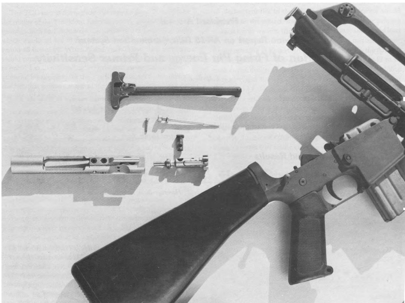
137. An early Colt model (6)02 (XM16E1) showing the bolt closure and modified charging handle contour, but still fitted with the early chromed bolt and original "heavy" firing pin.
