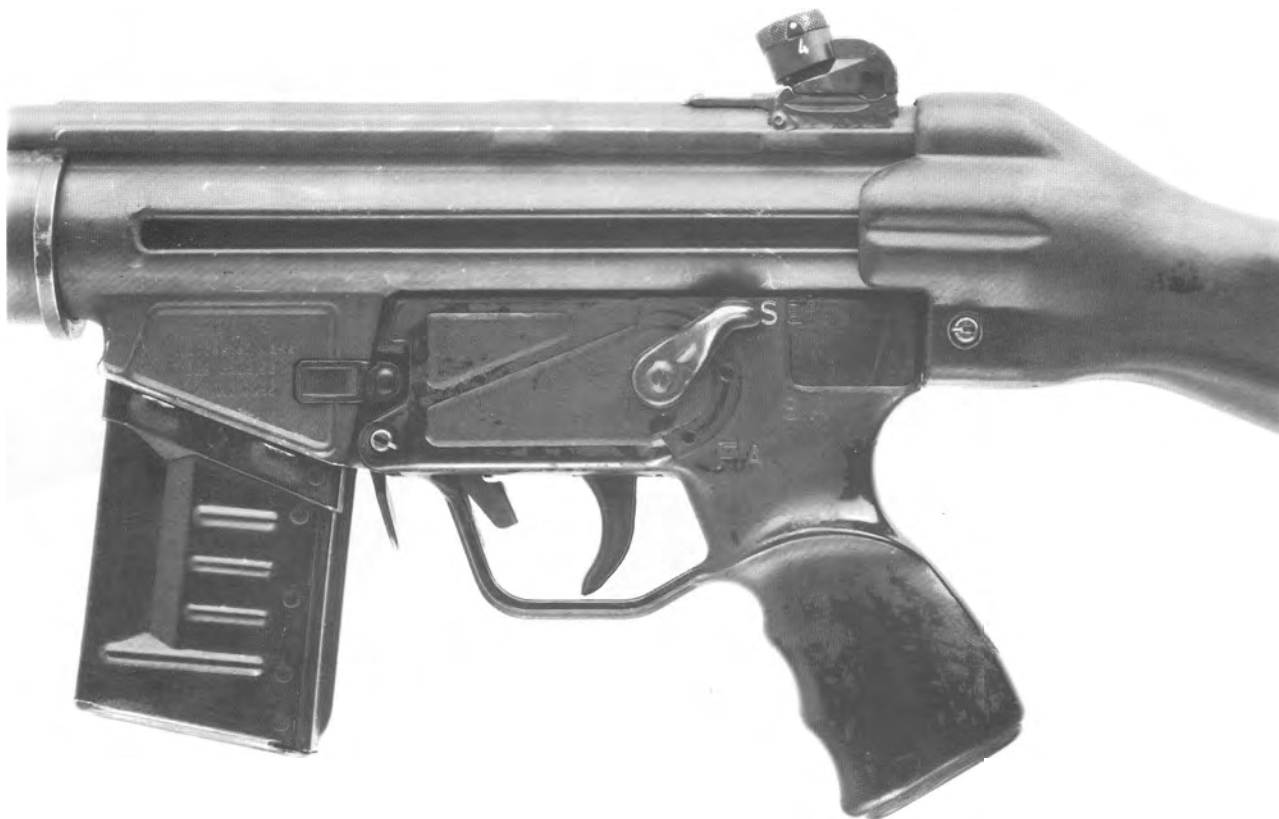
196. Receiver closeup of the 5.56mm caliber HK33, disguised as the "H&R T223" for the SAWS trials. Note the selector markings: "Safe: S.A; F.A".
