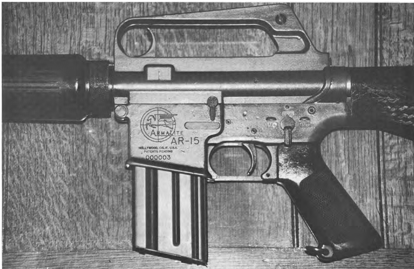
88. A closeup view of the receivers, left side, of the earliest ArmaLite AR-15s. Although serially numbered earlier than no. 000012 (fig. 75), various modifications, such as those recommended after the initial Infantry Board trial in March, 1958 have been made to both weapons. Rifle no. 000002 (above) has an experimental grooved slip ring and hence a two-
