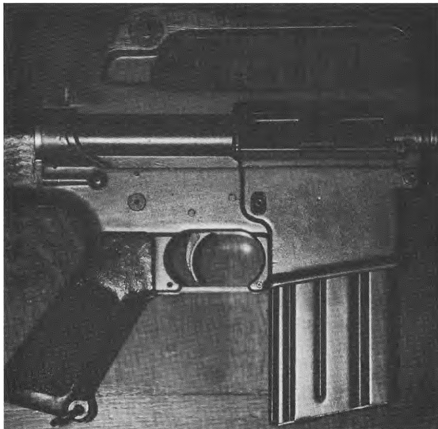
89. Closeup of the two receivers, right side view. No. 000002 (above) with modified charging handle. Both weapons feature woven fiberglass buttstocks, pistol-grip sling swivel, and the original 25-round magazine.
